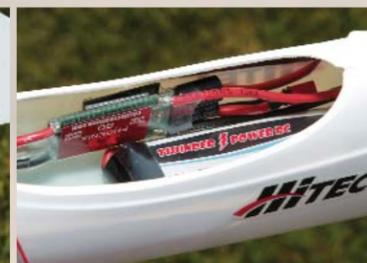
The forward hatch has plenty of room for installing the flight batteries. I am using the Thunder Power G-4 Pro Lite 3S 2600mAh pack and it seems a perfect combination of light-weight efficient power. Left: There's plenty of room for the
