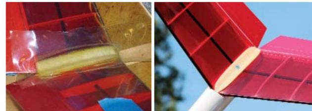
**I protected the tail surfaces with plastic film, and then used them as a mold to lay up the clamping plate for the V-tail. 30-minute Z-Poxy and a few layers of 1.5 ounce fiberglass cloth worked wonders. After a bit of trimming, sanding and drilling a hole for the hold down screw, the clamping plate is complete.**
