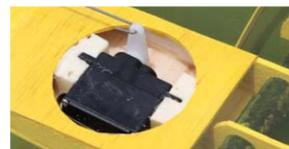
**The aileron and flap servos mount in the wing with traditional vacuum formed drag covers. I mounted the servo blocks with 30-min. Z-Poxy and secured the servos with Zap Goo. The kit includes pushrod hardware, but I opted for a direct wire linkage. I used Hitec HS-82MG servos for the flaps to prevent stripping gears when landing.**
