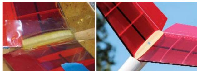
I protected the tail surfaces with plastic film, and then used them as a mold to lay up the clamping plate for the V-tail. 30-minute Z-Poxy and a few layers of 1.5 ounce fiberglass cloth worked wonders. After a bit of trimming, sanding and drilling a hole for the hold down screw, the clamping plate is complete.
